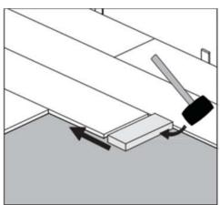
Step6: Attach a scrap piece of floor to bridge gap between ends of planks. Tap end of plank with hammer and tapping block to lock ends of planks together. Remove bridge and continue towards wall until installing the final plank in the row.
