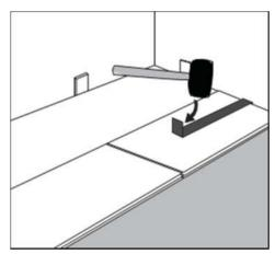
Step7: Use hammer and pull bar to lock final piece in row. Insert spacer at end of row. Continue installation to final row.
