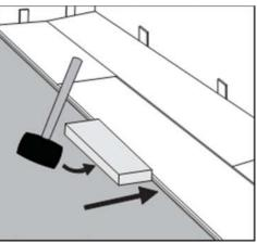
Step5: IMPORTANT! Use hammer and tapping block to tap long edge of plank to ensure a tight fit. Any gaping can compromise the locking system!
