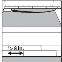
Step3: Use leftover plank from first row as starter for second row. There must be at least 8" between plank end joints on adjacent rows.
