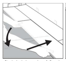
Step4: Lock long edge of floor by inserting tongue into groove at an angle and drop in place. Slide plank toward end of previously installed plank until the tongue just touches the groove.
