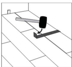
Step8: Use hammer and pull bar to lock long edges of planks on final row.
